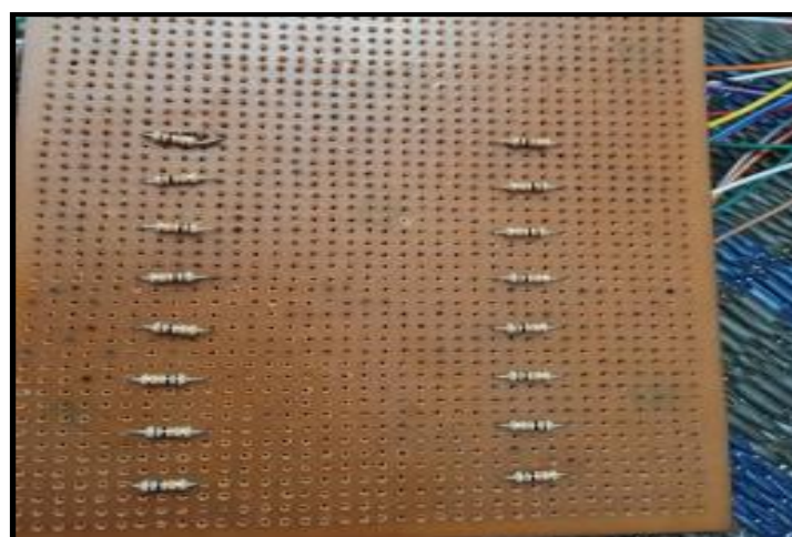
Figure 2. PCB and resistor connected with Arduino mega and power supply with the help of jumper wires
